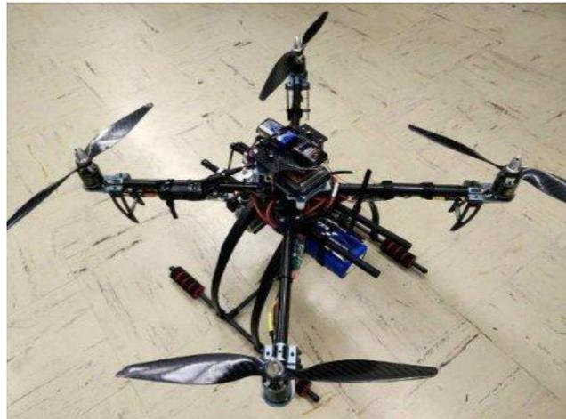
**Figure 2. Assembled quadcopter test bed.**
