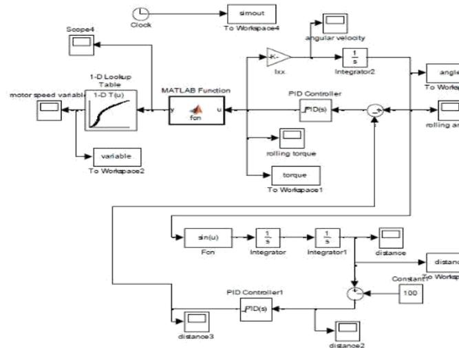
Figure 1. Combination of the rolling controller and the acceleration controller
